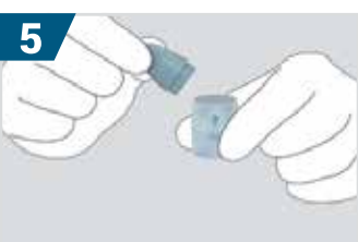
Remove the grey cap to reach the cover screw or the healing abutment.
